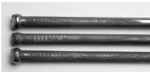
Product F severe tarnishing and surface oxidation, limited pitting
