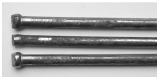
Product A significant corrosion, oxidation and pitting
