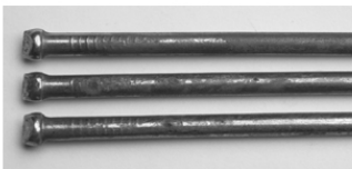
Product W Severe pitting and surface oxidation in parts
