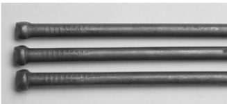
Salshield Rusteze No pitting or signs of corrosion, tarnished
